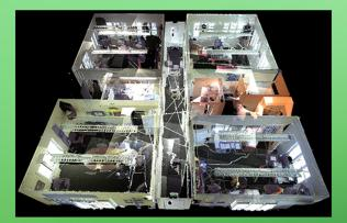
Ground-based LiDAR or static terestrial LiDAR, 3D laser scanning technology gives Frontier Geospatial the ability to quickly and safely collect spatial data for a site, structure or objects.
